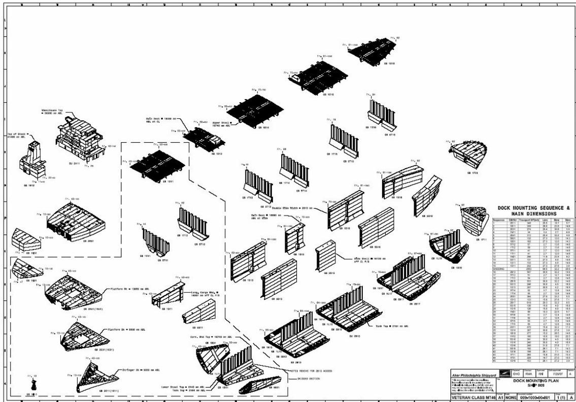
Fig. 8 - APSI Block Breakdown
