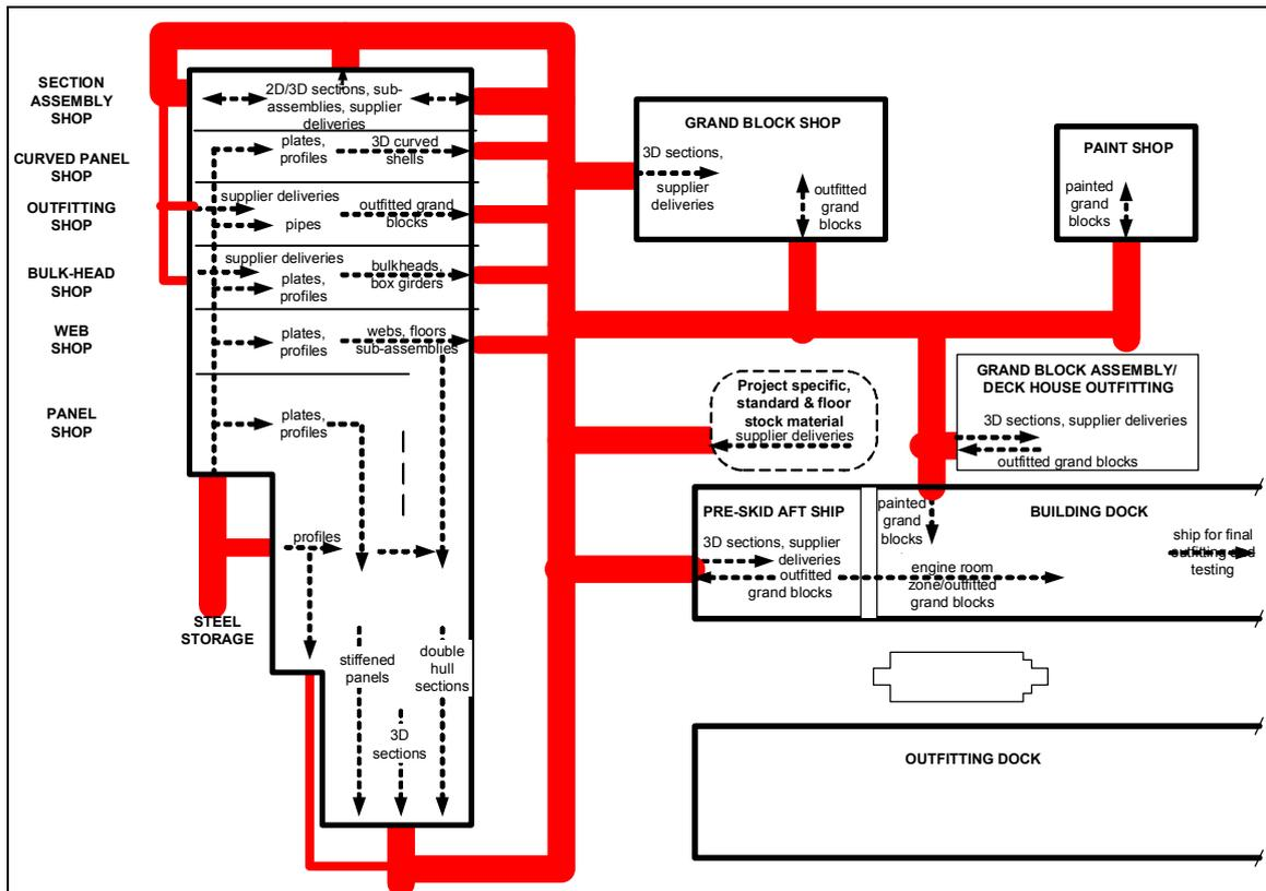
Fig. 7 - APSI Steel Handling Process
