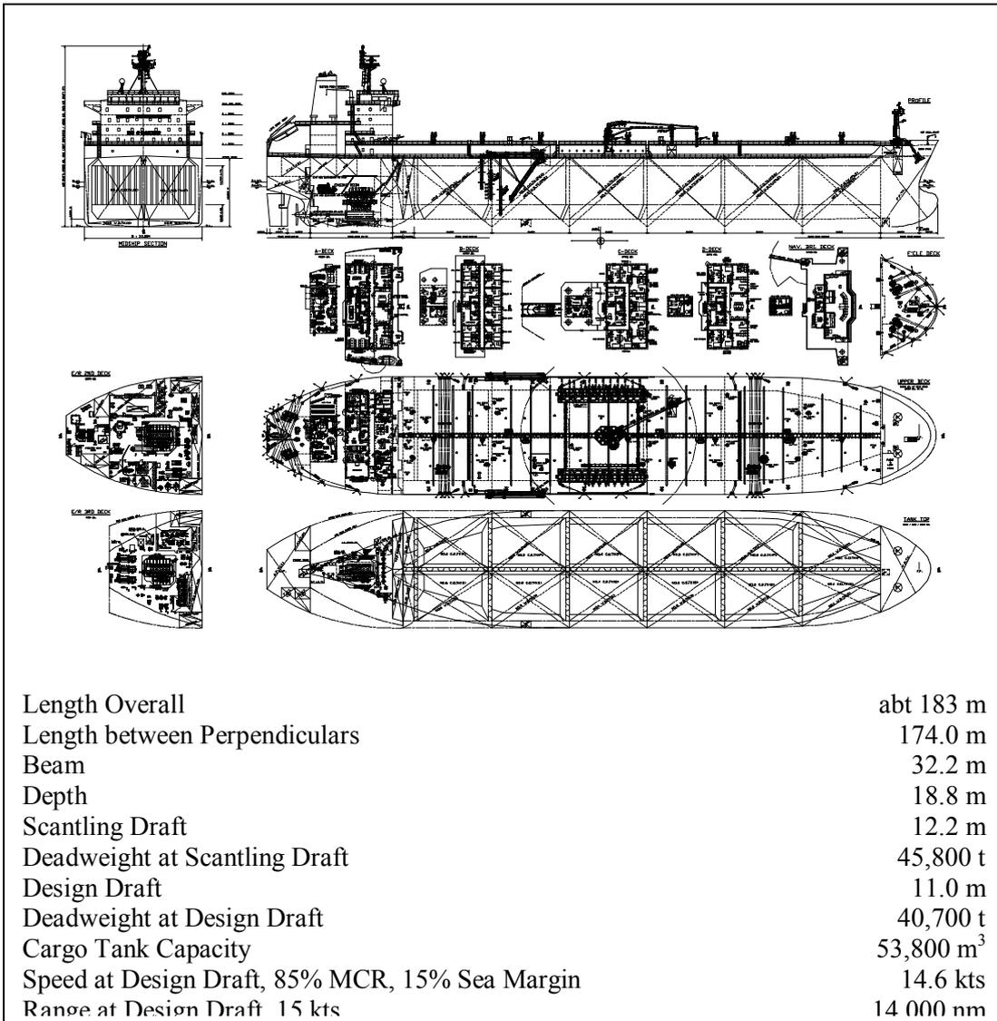
Fig. 4 - General Arrangement and Particulars
